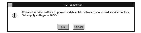
When external power is connected and user selects Yes to continue, the application displays the **Energy Management Calibration** dialog box:
